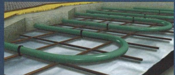
Radiant Floor Heating
