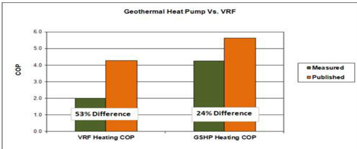
Note that for both heating and cooling, the VRF system's measured COPs and IEERs are roughly 50 percent less than the published data. For the water source heat pump system, the differences are significantly smaller and to be expected when system energy transfer – pump horsepower – is accounted for.
