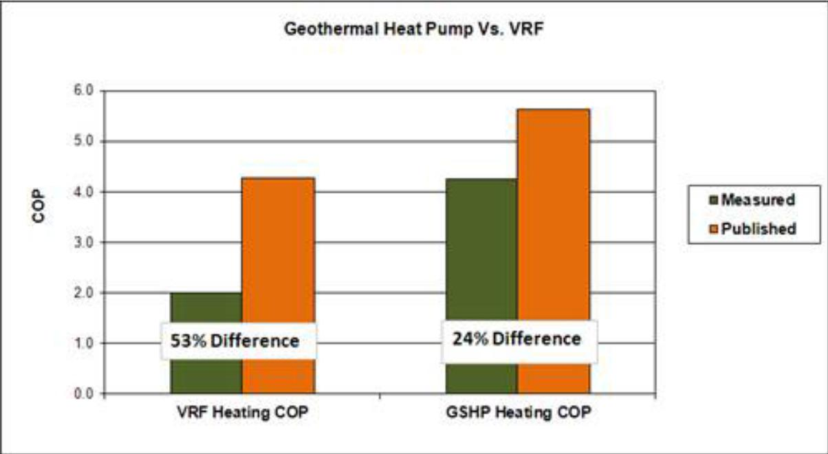
Note that for both heating and cooling, the VRF system’s measured COPs and IEERs are roughly 50 percent less than the published data. For the water source heat pump system, the differences are significantly smaller and to be expected when system energy transfer – pump horsepower – is accounted for.
